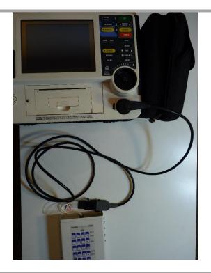
3. Connect the Pads to the **black** cable which comes out of the other end of the rhythm generator.
